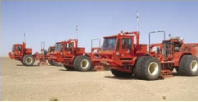
Veritas buggy-mounted vibroseis units explore for oil and gas in the deserts of Oman.
