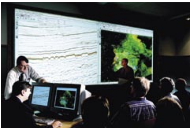
Significant seismic imaging advancements from time migration methods to pre-stack depth migration and wave equation migration are reducing finding and producing risks by providing interpreters with a clearer view of the reservoir.
