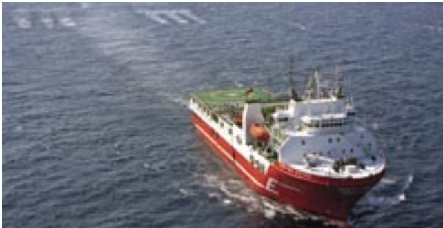
The SR/V Veritas Viking conducting a 3D seismic survey offshore eastern Canada
