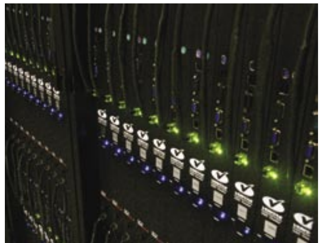
Cluster CPUs with new 64-bit Opteron processors are significantly reducing time-to-solution on processing large 3D data volumes.
